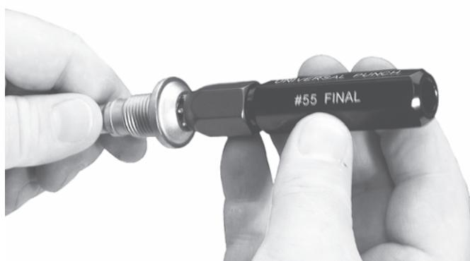
**Final Plug Gage:** This gage is single ended. Generally used for inspection of finished products, the Final Plug Gage is used to check acceptance of a drive form by representing the minimum form size allowable after plating. If the Final Plug Gage does not enter the form then the form has likely been coated past allowable limits during plating. For acceptance of the part, the Final Plug Gage should fully enter the screw form to its complete depth.
