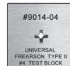
Test Blocks Are Heat Treated, Thermally Stabilized, And Surface Treated To Provide Additional Wear To Maximize Gage Life. Long Form Calibration Certificates Provide Dimensions And Tolerances To Specified Standards And Are Traceable To (N.I.S.T) National Institute Of Standards & Technology.
