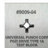
Test Blocks Are Heat Treated, Thermally Stabilized, And Surface Treated To Provide Additional Wear To Maximize Gage Life. Long Form Calibration Certificates Provide Dimensions And Tolerances To Specified Standards And Are Traceable To (N.I.S.T) National Institute Of Standards & Technology.
