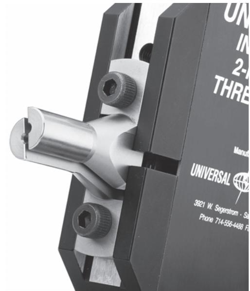
**INTERNAL GAGING ELEMENTS-** For measuring Pitch Diameter use single gaging elements "Cone & Vee" design. For measuring Functional Size use full form elements. For measuring Minor Size and Circularit y use plain elements. For Special Thread Elements priced on request.
